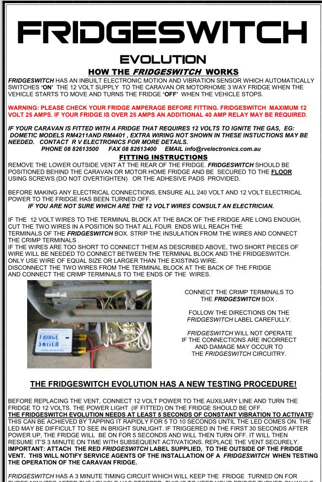
*FRIDGESWITCH* HAS A 3 MINUTE TIMING CIRCUIT WHICH WILL KEEP THE FRIDGE TURNED ON FOR THREE MINUTES AFTER THE VEHICLE HAS STOPPED. THIS IS TO KEEP YOUR FRIDGE TURNED ON WHILE YOU ARE STOPPED AT TRAFFIC LIGHTS.
